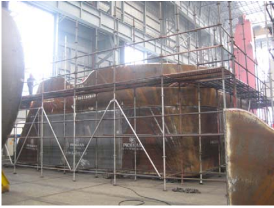
Huisman, building transition part crane base
