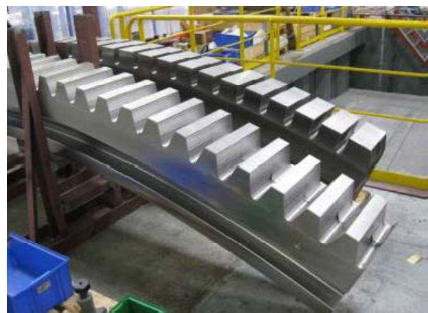
Huisman, pre-machined bearing parts
